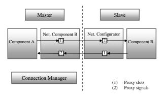
Figure 6. Remote connection between components in ARCS (Master-Slave)
