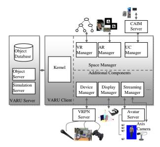
Figure 4. VARU main components
