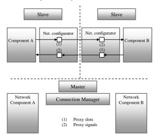
Figure 5. Remote connection between components in ARCS (Slave-Slave)
